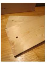
3. On the opposite end from the large hole, drill two pilot holes using the I/8" drill bit. They should be 3/4" from the bottom and side edges.
