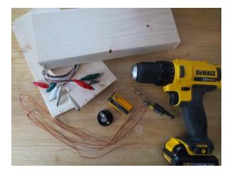
2.. On the 2 pieces of I"x 4"x 8" mark out a whole on one end of both pieces that is approximately in the center of the wood and I " away from the top edge. Using the drill, and the 3/16" drill bit, drill out both holes.
