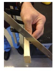
5. Using the piece that you just cut off lay it on top of your main board 1" from the angle cut end. Draw a straight line across your
