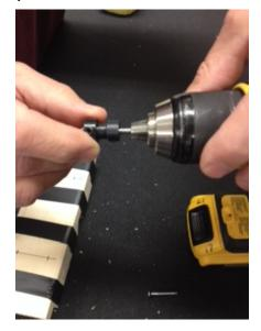
12. Drill each hole approximately ¾" deep. Be sure to hold the drill at a
