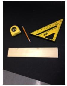
2. Using your tape measure, from the end of your board measure in 2 ½" and draw a line using your pencil. Ensure the line is drawn across the entire width of the board – use your speed square to ensure your
