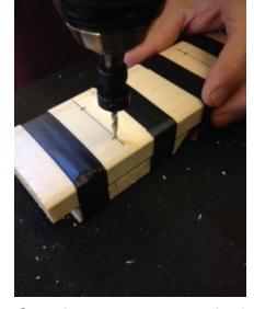
13. Switch out the drill bit for the counter sink drill bit and drill each of
