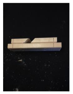
16. Carefully clamp your project to the table and cut off each of the waste ends.
