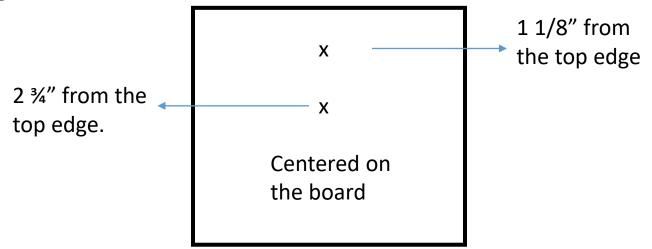
15. Again using your tape measure and speed square find the center on the edge of your roof piece. Do the same on the back side of the main post of
