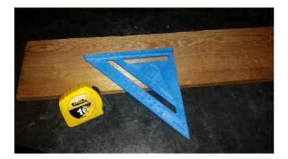
12. Using the tape measure – mark a line  $5 \frac{3}{4}$  " from the end of the board. With the speed square mark the line across the entire board.
