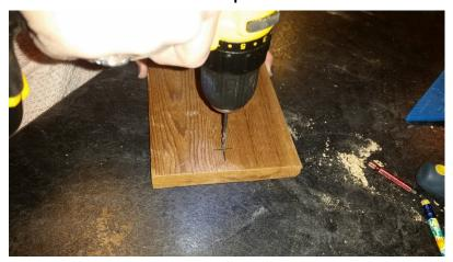
25. Using your countersink bit. Drill out your two center holes on the back side of your board.
