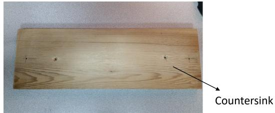
26. Turn the board over and counter sink each of the holes at either end of your board.
