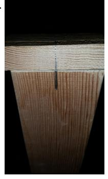
17. Use a 1/8 " drill bit in your cordless drill, and drill through the roof into you body the length of your drill bit. You will need to hold your pieces firmly in place. – This step is best done with a partner.
