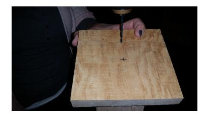
18. Using your counter sink drill bit on the roof piece, drill out both holes. – This will provide a divot for your screws to fit flush with your roof
