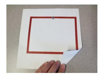
3. Peel backing off of the conductive tape and place on the paper template starting on the positive side of the circuit. Smooth the tape down as you go & stop just before you get to the corner.
