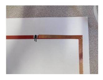
6. Repeat steps 3-5 beginning at the Negative side of the LED location. This side of the circuit has two corners that will need to be folded carefully into the 45° angle.
