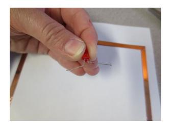
10. Place the LED onto the paper template as indicated and secure in place using scotch tape on either side.
