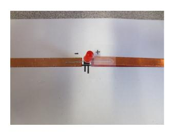
II. Place you battery on the Negative circle and fold over the corner with the Positive circle. This will light up your circuit, The paper fold becomes the switch that completes the circuit.
