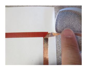
5. Continue to smooth the tape down as you get to the LED symbol, then cut or tear the conductive tape to complete this half of the circuit,
