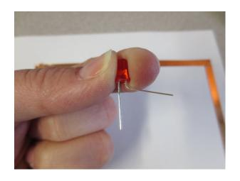
q. Carefully bend the negative leg of the LED, in the opposite direction.
