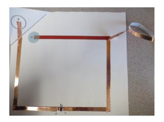
7. Continue to smooth the tape down as you get to the battery location, then cut or tear the conductive tape to complete the 2<sup>nd</sup> half of the circuit,
