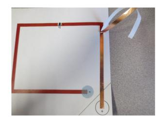
4. Fold the conductive tape over on itself and press down to make a 45° angled corner.
